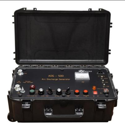
Arc Discharge Generator ADG-500 is a 10kV/500J Surge generator with built-in ARM (aka SIM/MIM) and ICM (aka WAVE) fault location modes.
