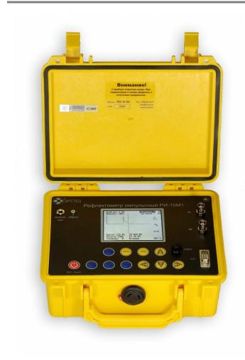
**TDR RI-10M1** – TDR cable fault locator, designed to determine the nature and location of the irregularities and damages of the cable line ((opens, shorts, wet/corroded splices, water in the cable, load coils, bridged taps, unknown splices, splits and re-splits, capture intermittent fault etc.)
