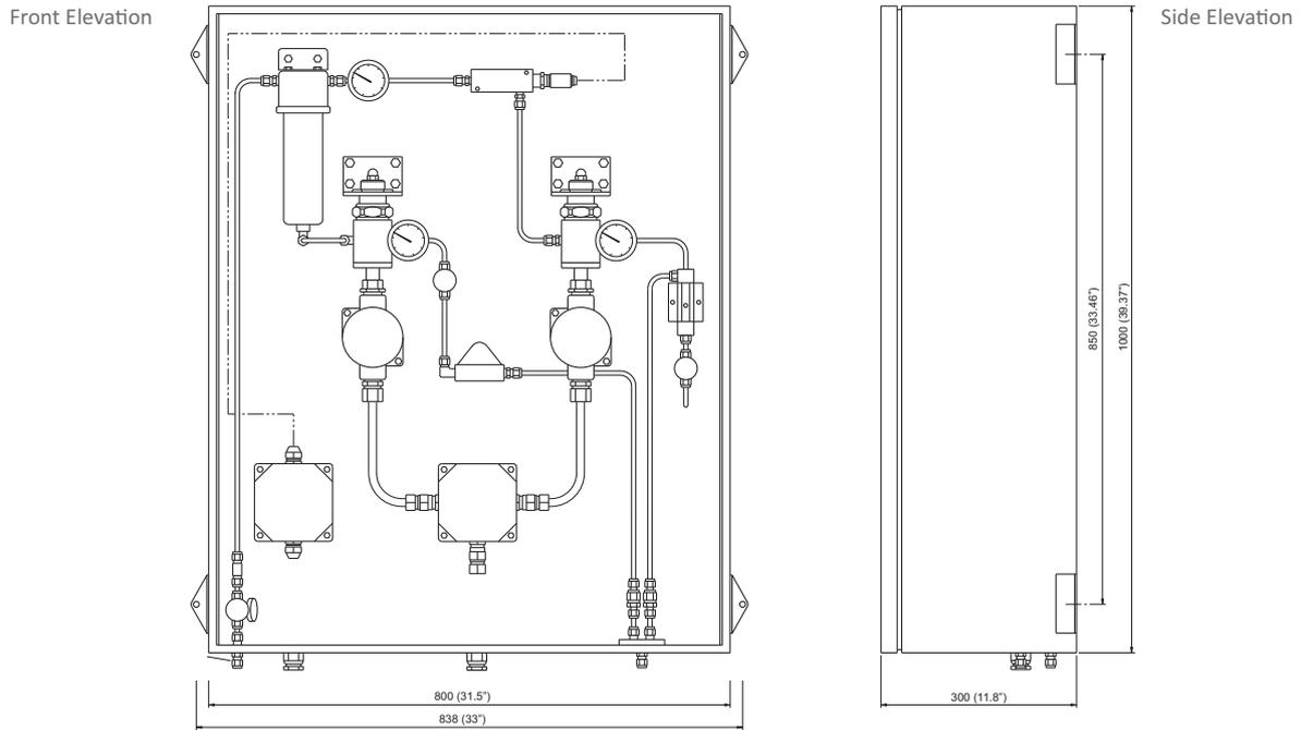
The heated regulators incorporated in the system can be installed for 115 VAC or 230 VAC operation, as specified on order.
