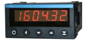
The linearizing is in a table format and the points can be entered from the keypad or from a PC. The Soft manager Orbcom for Windows supports the entry. With the keyboard the menu can be opened. The menu contains Scaling, Preset, Filter, Sampling Time, Reset Time, Password, Analogue Output, Serial Data Ports and Set Points. The Counter function can be set for Quadrature Counter, Up-Down Counter or Tachometer.
